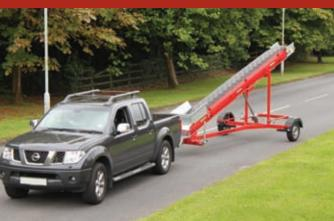
Along with many other applications this conveyor represents the ideal solution for dosing steel fibres and ad-mixtures into concrete trucks. The 'EASIVEYOR' which weighs less than 600kgs can be easily towed from depot to depot or from site to site behind standard vehicles fitted with a 50mm ball hitch. The conveyor is based on an Easikit 450 conveyor 6 metres long and is supplied complete with a 110v Motor pre-mounted and wired with plug ready for connection to power supply.
