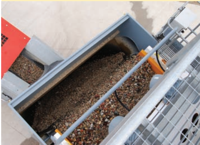
Holcim Chepintsi scrubbed material discharged from Rotomax and dewatered, factory Rotomax shaft from left side showing fan arrangement of paddles
