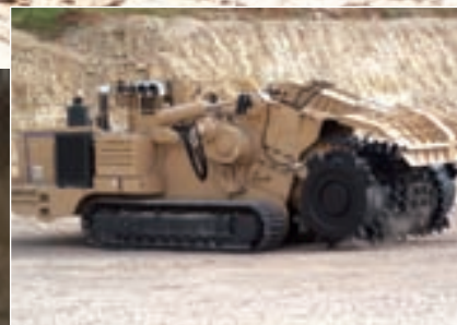
The Rock Hawg planes out a haul road
