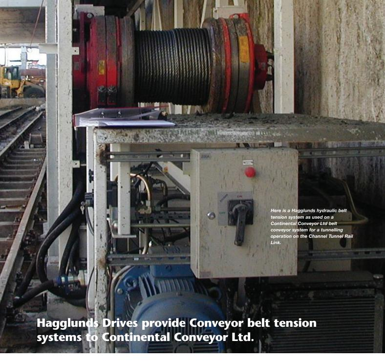
The essential requirements for a large conveyor belt tension system is to provide an accurate set slack side tension which is consistent in all conditions whilst the conveyor is running. This prevents sag in the return belt and loss of troughing contour in the carrying strand of the belt. A fast response time is important to eliminate transient peaks during changes in the conveyor loadings absorbing the elastic belt stretch.
