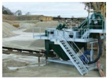
With a busy operation of this nature it was of prime importance that the processing plant operates efficiently; however it had become apparent that the existing screw/bucket dewatering unit was losing fine sand to the settling lagoons. It was therefore decided after consultation with Finedoor that it would be beneficial to replace the inefficient unit with a modern hydro cyclone sand treatment unit.
