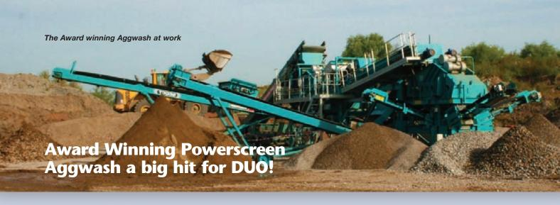
The Powerscreen® Aggwash was voted the winner of the Series **Innovation Category at the 2010** World Demolition Awards. The new concept is a development in mobile wash plant which unifies for the first time rinsing, screening, scrubbing and sand washing capabilities on a single transportable chassis.
