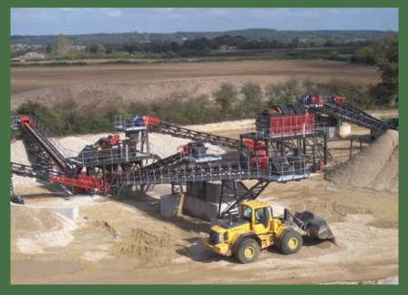
wide x 500/3-ply all-nylon belts with rubber covers, supplied by RAP Conveyors. The conveyor drive shafts run in INA FAG self-aligning ball bearing plummer blocks, while the belts themselves travel on 102mm diameter three-roll, equi-length, drop-in idler sets with sealed-for-life bearings supplied by Rulmeca UK Ltd. Scraper sets from RH Conveyor Services are fitted under all head drums for belt-cleaning purposes.
