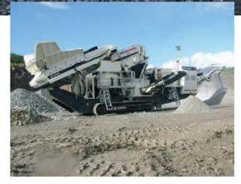
The hydraulically adjustable feed conveyor allows the machine to be operated using either the innovative prescreen system or if required by feeding directly into the cone.
