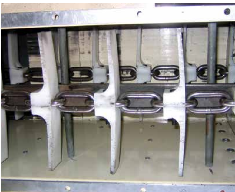
Bolt-N-Go System Round Link Chain Application on a Conveyor
