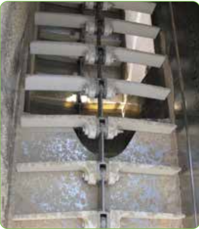
Feed Mill Application using Bolt-N-Go Chain with Nylon Flights
