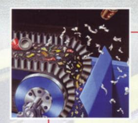
An Eddy Current Separator basically consists of a short belt conveyor with its drive at the return end. Inside the delivery pulley a rotor fitted with magnets spins at high-speed generating a high frequency alternating magnetic field. In a similar manner to electric motors the alternating magnetic field sets up an electric current in conducting metals within its influence, which in turn produces a magnetic field opposing that of the
