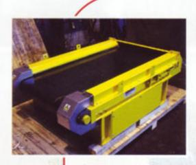
Master Magnets ECS designs incorporate the latest generation neodymiumiron-boron rare earth magnetic elements to give the high field strengths necessary for efficient separation. Careful design of the rotor within the outer pulley shell ensures that the product is as close as possible to the magnets, as does the selection of high quality thin section conveyor belt.
