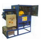
conductive/non-conductive separations utilising the differences in surface conductivity of granular particles.
